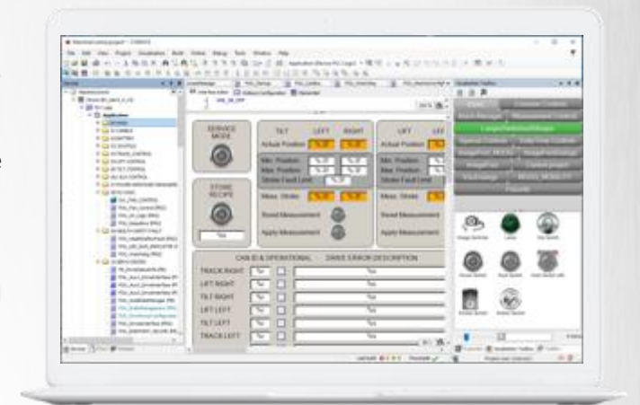
Figure 1 | CODESYS IDE: Device Tree and Display Editor
